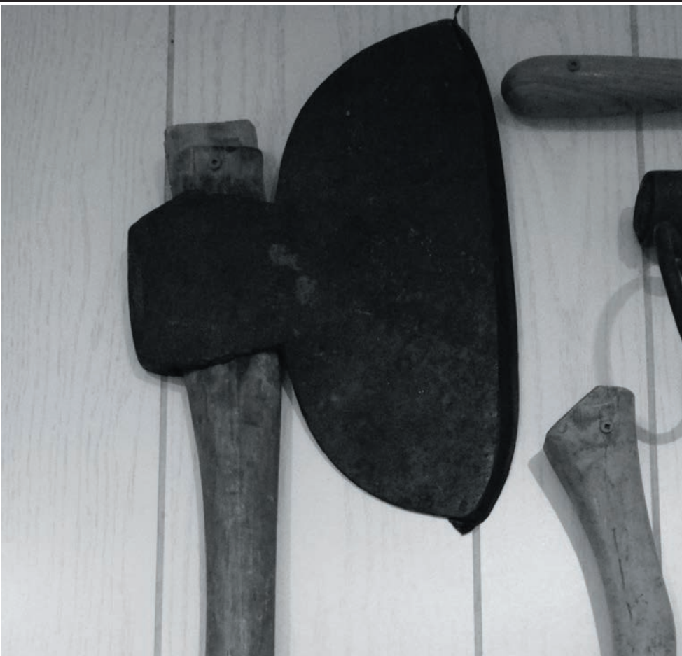
You can see here that the broad axe and handle are flush with the wall. There is no bevel on the flat side, but you can see the sharp bevel on the cutting edge. A sharp axe and strong accurate strokes were key to creating square timber - not an easy skill to acquire.
