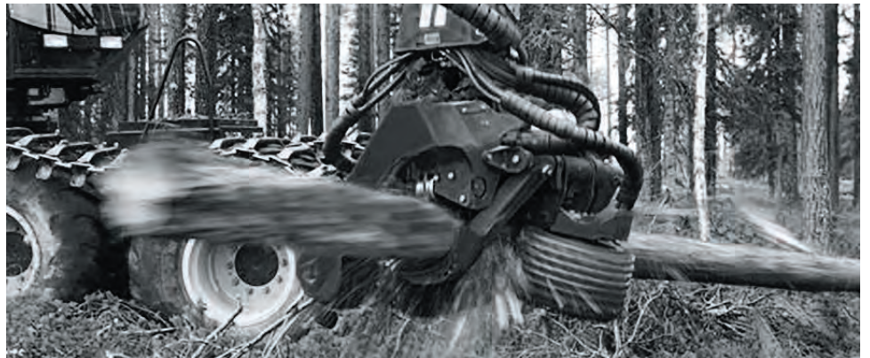
The Valmet, invented in 1984 in Finland, revolutionized logging. Felling, delimiting and bucking - all with one grip.
