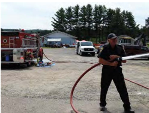
Water from the collapsible reservoir is pumped into the fire truck then out again at high pressure while the tanker, or pumper truck does another run for water at a nearby lake or river.
