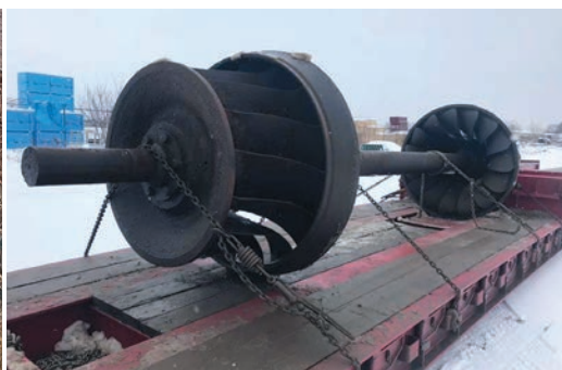
Work to dismantle and expand the OPG Generating station in Calabogie continued over the winter. Turbines that have been operating since 1914 were removed and shipped out. Pics by Nick Tourangeau and Jeff Levesque
