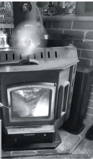
Thermocouplers use the difference between the hot stove and the cooler top part of the fan to generate electricity that drives them.
