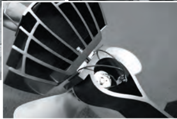
Thermocouplers use the difference between the hot stove and the cooler top part of the fan to generate electricity that drives them.
