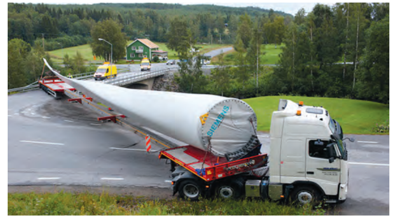
Delivery of Wind Turbine parts in Sweden. About 8 trips are needed for each wind turbine and every step of the slow journey must be carefully planned and permitted. (image statkraft.com)
